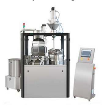
NJP-3800D Automatic Capsule Filling Machine adopts butterfly valve-type powder feeding, and is very suitable for drug powder with poor liquidity, including Chinese herbal medicine and Chinese patent drug, due to that its vibration unit equipped will force the powder to run down, which has solved problem of failing to feed in powder that often happens in the traditional screw feeding device because of the poor liquidity of powder.
