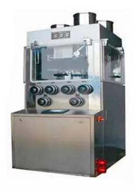
ZPW three layers Multi-functional Tablet Press has a wide scope of application. It is applicable not only to the pharmaceutical and foodstuff industry but also the chemical, ceramic, electronic and battery industry for pressing the various kinds of granular materials into tablets.
