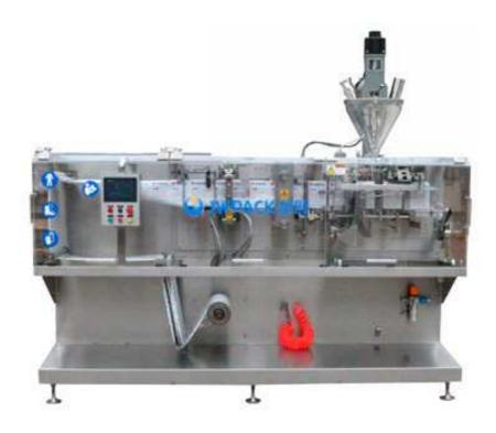
DXD-130D Automatic Horizontal Pouch Packing Machine contains motor film-releasing, film forming, bottom sealing, vertical sealing, cutting, filling, pouch transferring and top sealing. The cams on the main shaft finish the coordinated action driven by the motor and the encoder on the main shaft feedback the position single. Under the control of the PLC, it realizes the function of film roll—film forming—film in-shape—powder filling—sealing—finished products transferring.
