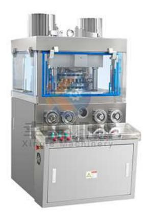
This machine is a double-press type, continuous automatic tablet press for pressing granular raw materials into tablets. It is mainly used in pharmaceutical industry and also the chemical, food, electronic, plastic and metallurgical industries.
