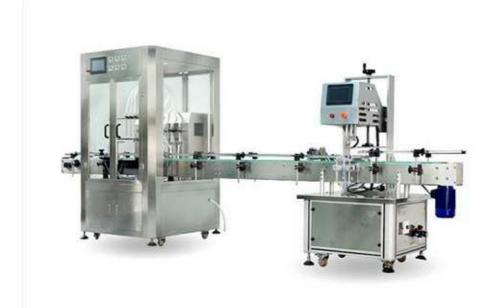
High precision automatic 6 nozzles filling machine - it is a mechanical rotary, atmospheric pressure filling, metering plunger cup quantitative filling valve
