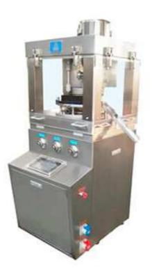
Single-pressing type and single-sided tablet discharging. It uses IPT punch to press granular raw materials into round tablets and special-shaped tablets of various specifications. It belongs to small production equipment and also used as pilot test equipment.
