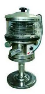
The LQ-CFQ deduster is an auxiliary mechanism of high tablet press to remove some powder stuck on surface of tablets in pressing process. It is also equipment for conveying tablets, lump drugs, or granules without dust and can be suitable for joining with an absorber or a blower as a vacuum cleaner. It has high efficiency, better dust-free effect, lower noise, and easy maintenance. The LQ-CFQ deduster is widely used in pharmaceutical, chemical, food industry, etc.
