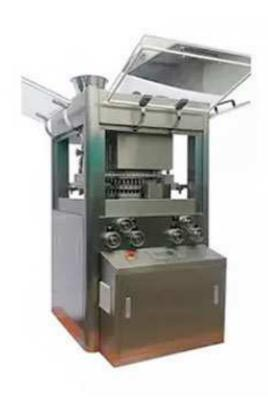
This is a new developed sub-speed rotary tablet press machine with high working capacity, heavy working pressure to compress the granule materials into various tablets such as round shape tablets, irregular shape tablets and even ring shaped tablets, applied widely to the industries of pharmaceutical, chemical, foodstuff, and electrical etc.
