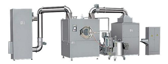
The Film Coating Machine can be used for coating various tablets, pills and sweets with organic film, water-soluble film and sugar film, etc., in pharmaceutical, food and biological industries. It is noted for its high efficiency, low energy consumption and space-saving qualities.
