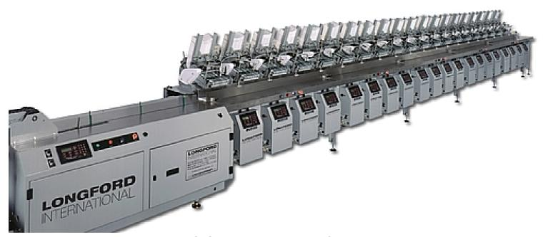
Design/build turnkey collator, fulfillment system that feeds, collates, stacks maps (charts) for fulfillment to pilots and airlines. Needs to run 4500 pph. Provide twenty (20) station collator that feeds, counts collated the charts, stacks in neat take-away piles for further packaging and marketing.
