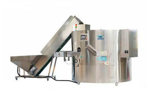
This machine adopts advanced technology, PIC intelligent control, and this machine does not change the mould can arrange for size similar and different shape plastic bottle, could use detergent square bottle or bottle with handle, and such as shampoo bottles, soy plastic bottles.
