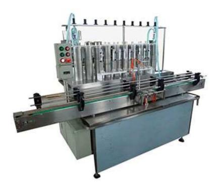
This chemical product filling machine is the main equipment of liquid production line, and it is mainly used for liquid filling of 100ml-500ml glass or plastic bottles. Its main component is cylinder filling machine.
