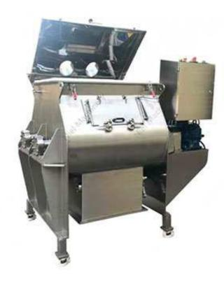
Double shaft paddle mixer machine is also called non gravity mixer machine or twin paddle mixer, it is widely used for drying and mixing of dry powder mortar, chemical, pesticide, detergent, pigment food, monosodium glutamate, milk powder, salt, feed, chemicals, ceramics, plastics, rubber additives, and other powders.
