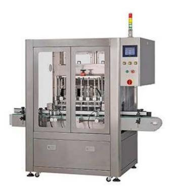
Automatic Gear Pump Liquid Filling Machine FP-465 is designed and engineered to produce outstanding quality and precision filling suitable for various products like shampoo, hot sauce, lubricant oil etc. FP-465 can also replace piston or peristaltic module for the flexibility of filling demands.
