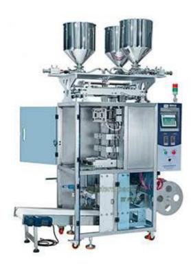
Shampoo pouch packing machine is suitable for automatic liquid of liquid, viscous body, paste and paste materials in food, chemical industry, medicine and other industries. Suitable for customers looking for Irregular Shaped.
