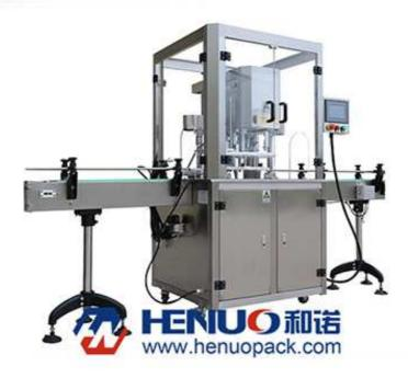
This machine is applicable for seaming the round can or jar with lid which is made of aluminum, tinplate and the other kinds of metal.
