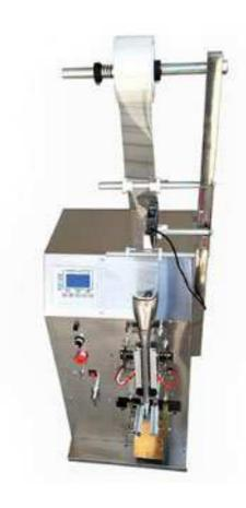
Automatic liquid quantitative packaging machine with double rod structure, which is reliable in performance, also has special adjusting structure deviates from the heart, can adjust the filling quantity when walking bag, on the species also have both quantitative pump and self-priming pump, the user can choose according to their own actual situation.
