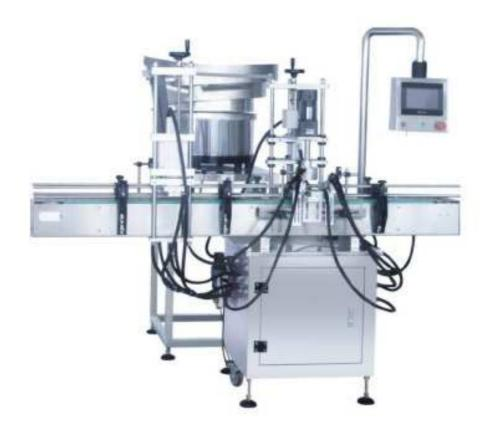
Designed for capping bottles with height 50 - 200 mm (can be customized) and diameter 35 - 70 mm (can be customized). Equipped with 1 capping head. To operate the machine needs compressed air supply with a pressure of 0.6 MPa.
