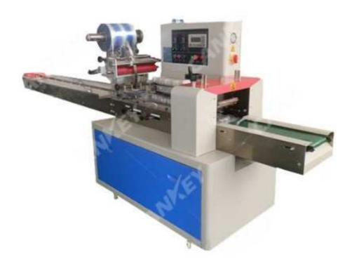
The automatic bread packing machine adopts servo control and introduces reciprocating end sealing and cutting technology. High speed, high precision, high stability. And the touch screen makes the operation simpler and more intuitive.
