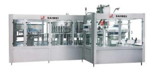
This machine is suitable for filling juice with pulp in both wide mouth and small mouth PET bottles. After washing, filling pulp, filling juice and then capping. The pulp is suspending and heterogeneous in the juice. Output is from 5000BPH to 30000BPH for choicest is the most ideal pulp juice filling machine.
