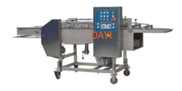
This Patty battering machine can offer an even coverage of the chicken (poultry), beef, meat, seafood, etc. by the batter curtain on the top and the dipping on the bottom. There is a blower designed to remove the excess batter before entering the next processing procedure of breading or predicting.
