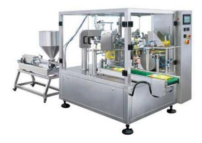
This line mainly use cylinder pump for feeding, it suit for all kinds of paste and liquid filling, such as juice, jam, ketchup, and shampoo etc.. and quite match with most premade bag shape such as doy pack bag or zipper bag.
