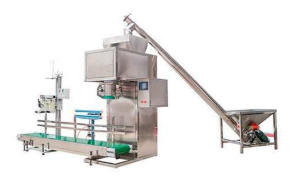
50 kg dry powder big bags filling machine net weigh auger filler is a new generation of smart Auger Filler Machine developed by Vtops Machinery. It using electronic weighing principle to weigh and fill materials. And the big bags filling machine adopts fast, medium and slow three-speed auger filling mode, with characteristics of high precision, high speed, and free dust pollution.
