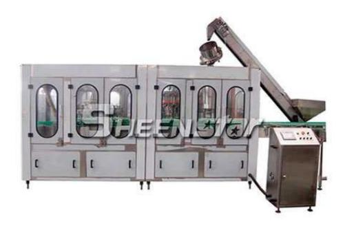
This carbonated drink bottling machine can produce 10000 bottles gas water per hour in 500ml glass bottles with crown caps.
