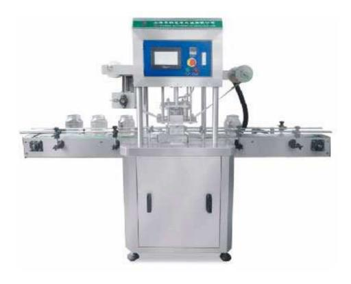
Auto Aluminium Foil Sealing Machine is specially designed for the bottle or jars heating sealing, to improve the shelf life of the products. Auto Aluminium Foil Sealing Machine with small size, easy to operate and maintain.
