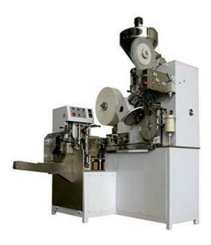
Tea bag packing machine Model DXDC8IV is our newest model, and features filling, heat sealing, threading, labeling and over-wrapping functions. Adopting sealing pads in place of the sealing rollers used in machines of previous generations, this new system greatly improves the machine's flexibility and enables use of different packaging materials. Main materials include paper/PE, plastic/foil/PE and plastic/PE.
