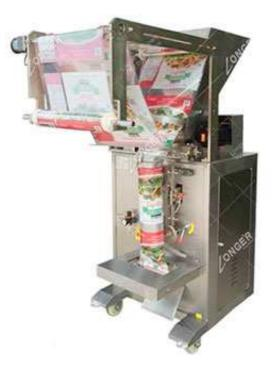
Turmeric powder packing machine is widely used for packing turmeric powder, pepper powder and other powder products.
