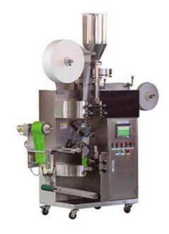
Our tea packing machine SPM-T100 is designed to packing filter tea bag with Envelope outer bag. The tea bag is formed in the first station and the outer envelope is simultaneously formed in the second station. The formed tea bag is then automatically inserted into the outer envelope and the outer envelope is sealed. This machine is suitable to pack Tea, Herbal products, Coffee.
