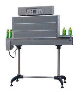
This series Bottle Labeling Machine are mainly used to shrink label of product in bottle shape, can shape or barrel shape with glass bottle, plastic bottle or paper cup. The label either on the top, in the middle, at bottom of bottle or wrapping the whole bottle is able to be shrank with different type model. It is widely applied in the industry of food, medicine, cosmetic and pesticide, etc.
