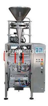
This Sugar Packing Machine is suitable for the suagr, salt and rice packing in pillow bag at laminated film or single layer PE film. The sugar packaging machine is equipped with volumetric cup.
