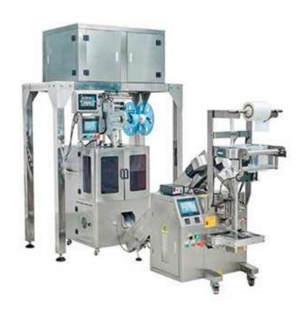
This is a scented tea triangle bag tea packaging machine, using nylon transparent film with thread and label as packaging material which have good perviousness and perspectives. It makes the tea leaves have enough permeability and space to allow the hot water to flow freely so that the tea products can release the fragrance when brewing.
