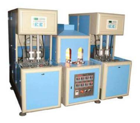
Semi automatic bottle blowing machine for PET PC bottle blowing the various shapes, volume from 50 ml to 2000 ml, the bottle blowing machine is widely used for blowing mineral water bottles, soda bottles, cosmetic bottles and bottles.
