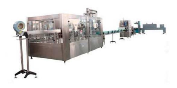
This Machine mainly used in the beer filling operations, the three function of bottle washing, filling and capping are composed in one body of the machine, the whole process is automatic, it is conveniently trunked to adjust the machine to fill various types of bottles, the filling operation is faster and more stable due to the advanced Germany filling valve technology. The famous brand programed controller (PLC) is adopted to control the machine runs automatically.
