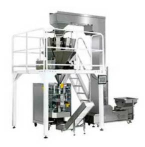
Suitable for packing granular, flaky, strip products, such as sugar granules, potato chips, shrimp chips, jelly, peanuts and so on.
