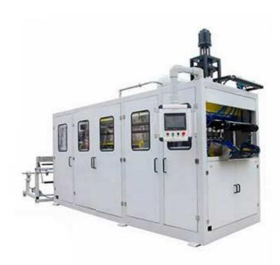
The Disposable Cup Thermoforming Machine is fit for producing PP, PE, PET, HIPS, GPPS and other plastic products, such as cup, box, bowl and so on. For example, milk cup, jelly cup, ice cream cup, one-off cup, instant noodle bowl, fast food box and so on.
