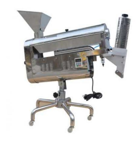
SPF15 Capsule Sorting and Polishing Machine. After polishing, that the capsule could enter into rejection system and choose the light filling, empty filling, fragment and separate of body and head through the airflow. It could be avoid contact of person and power and then make sure the quality of tablet. This machine is suit for all kinds model of capsule and capsule filling machinery.
