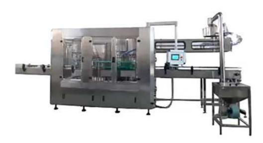
This series equipment is used to produce all kinds of carbonated drink contained in PET/Glass bottle, washing, filling and capping into one unit. It can be used for hot-filling production of different kinds of fruit juice, tea drink, etc. This series machine can be also used for the filling of purified and mineral water.
