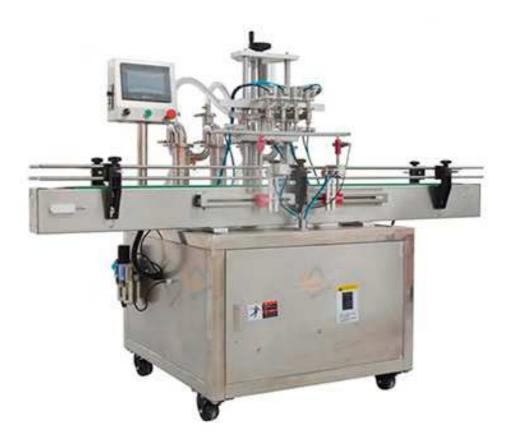
This is an fully automatic liquid filling machine with 4 filling head. It adopt the pneumatic driven cylinder dosing unit that Automatic suction and filling liquid item quantitatively. It is suit for low viscosity liquid item such as water, wine, alcohol, liquid detergent, juice beverages (such as tea drinks, soy sauce, jam vinegar) etc.
