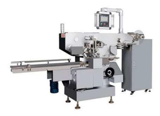
Model SL-SBZB450S used for aluminum foil packing style. The aluminum foil wrap the confection completely and highlight the shape of the confection very well.
