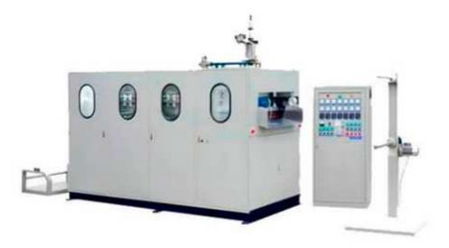
It's suitable for plastic sheet forming, such as PP, PE, PS, HIPS, PVC, PET, PVC, PLA. It can produce different kinds of cups, bowls, dishes, lids and boxes such as milk cups, jelly cups, one-off cups and instant noodle bowls.
