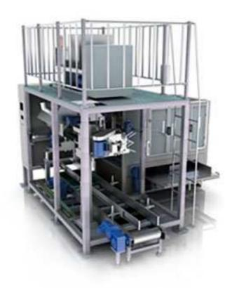
The automatic large package production line is composed of CML charging machine, DCML automatic bagging machine and DCML automatic sealing machine. CML charging machine has been listed in the catalogue of special equipment for civil explosion, and the latter has passed the appraisal of technical achievements.
