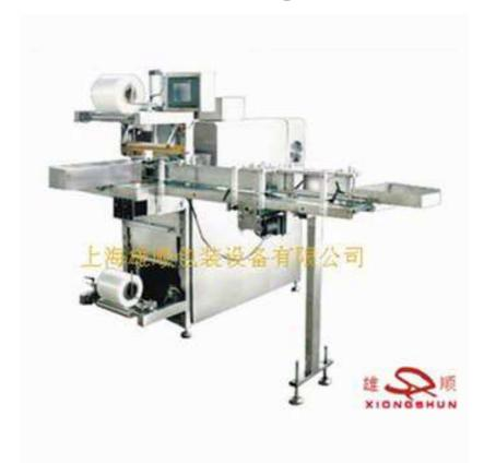
The machine is applicable to packing large injection, beers, drinking, and milk products, mineral water with one-row and multi-row heat shrinkage films. It designed with German advanced technology based on the European technology. And the electric components are all adopted the famous brands at home and abroad, which ensures the reliability of machine in running.
