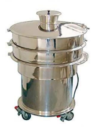
Vibro sifter is circular gyratory screens used to separate mass composition of solids, liquid from solid and for gradation of materials as per particle sizes Vibration is generated in three different planes along the vertical axis by means of a specially designed vibratory motor having off centered weights at the top and bottom end of the motor shaft.
