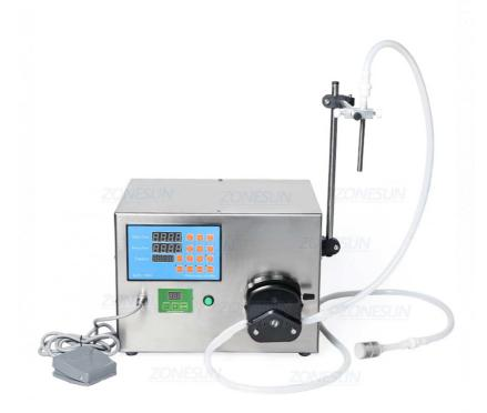
The main advantage of this machine is that the liquid will not pass through the pump during working. This ensure the cleanliness of the product. This machine can be used to fill essential oil, milk, beverage, solvent etc.
