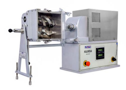
Laboratory Kneader is operating on the Z blade principal. It consists of two Z-shaped mixing blades rotating towards each other at different speeds which cut down substantially the required batch mixing time. The bowl and Z mixing blades are made of stainless steel. The bowl has an acrylic cover which allows visual observation of mixing and the above cover is having electromagnetic safety switch. The Laboratory Kneader is suitable for screwing on all main drive units.
