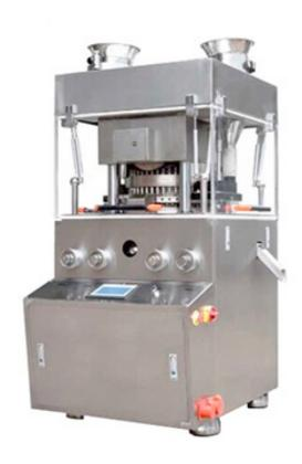
ZP Series is kind of double pressure type automatic rotation, continuous tablet machine. The particle pressure into a round, irregular, it can also be lettering, dual color. It is mainly used in pharmaceutical industry tablet production, at the same time, it is suitable for chemicals, food, electronic, and other industrial enterprises.
