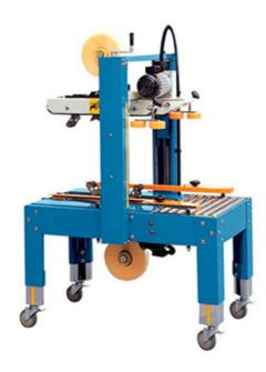
The CHS-6602 carton sealer is a semi-automatic manual adjustment carton sealer having top and bottom carton sealer. The CHS-6602 is easy to use and simple to adjust which enables any operator to start production just in Minutes. We have designed carton sealing machine according to the CE standard. 2' taping heads or 3' taping heads are according to customer requirements.
