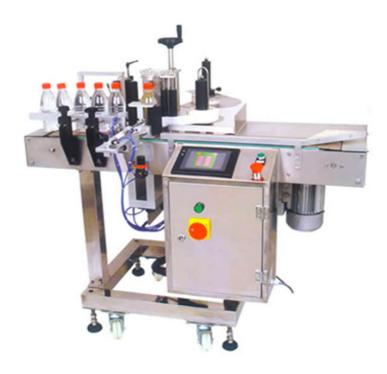
This machine is used for using most advanced touching type man-machine interface with English showing. The replacement of object does not need to move the electric eye. The circumference placard, makes two labels at the same time glues, also two label spacing may adjust at will; Also may attach the printer, the synchronization completes the label printing. It is suitable for processing the column object of the wines, food, cosmetics and medicines.
