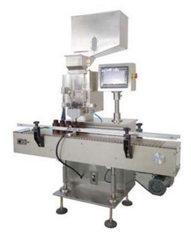
SSL-1A capsule counter is widely in small-scale production in hospital, pharmaceutical factory, R&D center for capsule counting. SSL-1A intelligent automatic capsule counting and filling machine adopts proprietary technology, PLC control, touch screen operating system. It can count and fill automatically with high accuracy. Feeding turntable, capping machine and labeling machine are available to connect to a line.
