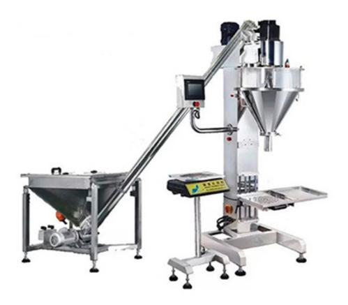
This machine is suitable for packaging fluidity Powdery product like milk powder, albumen powder, solid drink, white sugar, dextrose, coffee powder, rice powder, fodder, pharmaceuticals, agriculture pesticide, granular additive, dyestuff etc in bag, can, bottle package. Stainless steel design, in line with GMP standard, It can do measuring and filling work.
